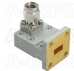
28WCAKM_Cu Right Angle Rectangular Waveguide to Coaxial Adapter 26.5-40GHz WR28 to 2.92mm Male
