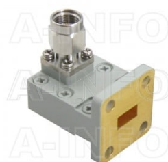
28WCA2.4M_Cu Right Angle Rectangular Waveguide to Coaxial Adapter 26.5-40GHz WR28 to 2.4mm Male
